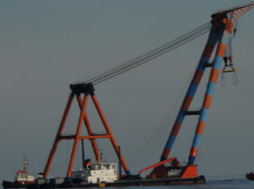
Crane ship Samson (860 tons capacity)
